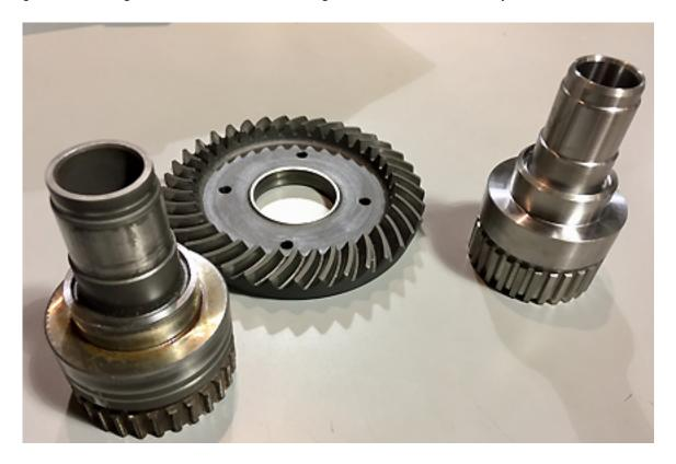
We've developed our own rotary welding fixture so that the new splines can be welded in place with clean, smooth welds.
