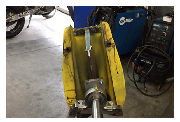
Rear Spline replacement for your 1970-1984 twin shock bike. As the miles go up the splines on the original rear drive go down. We now offer a stronger solution that will outlast your bike!
