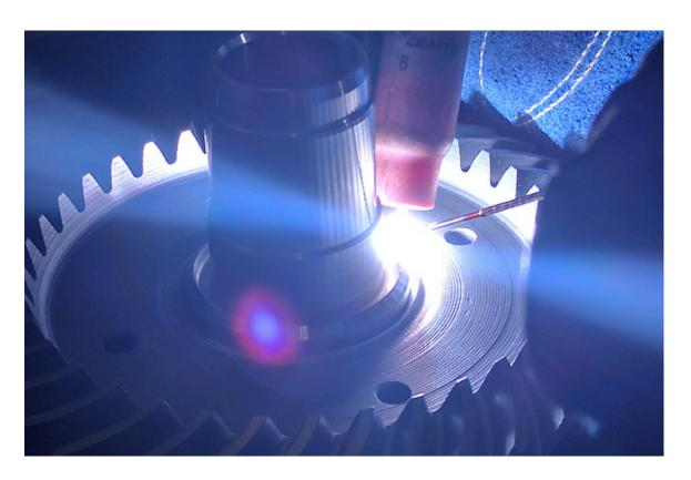
Our Miller Syncrowave 210 Tig welder does the work of joining the new parts.
